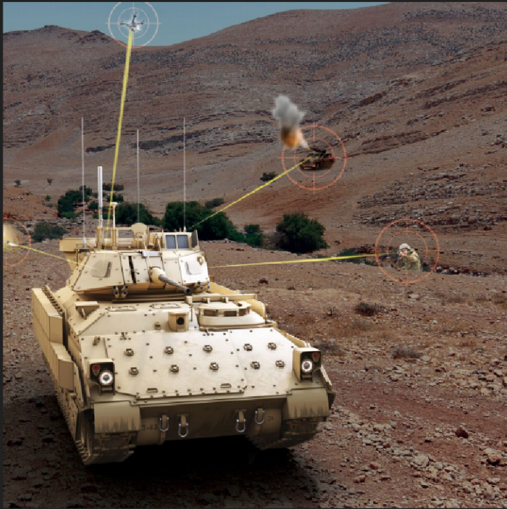
Stormguard, a radar for tanks and other land vehicles that performs surveillance and coordinates “counter-fire”
