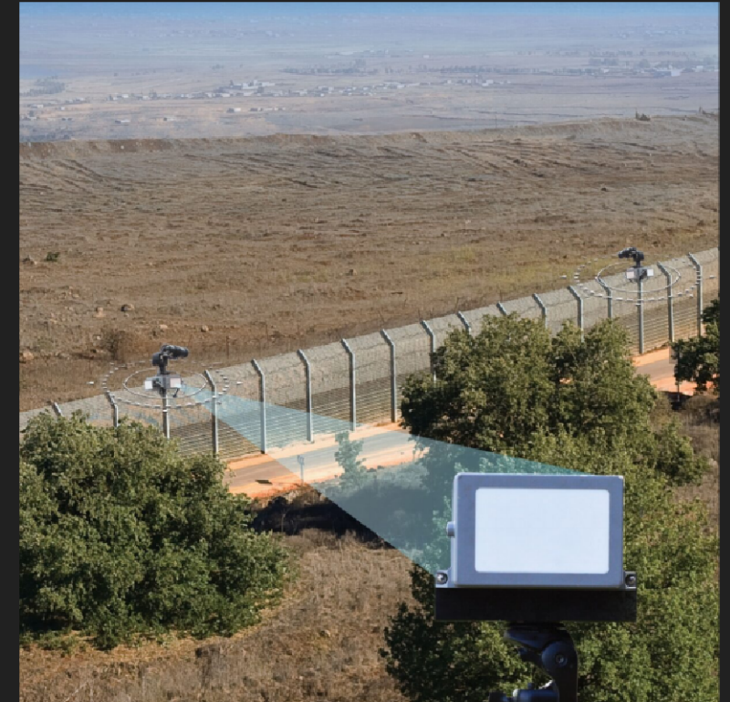
The Persistent Perimeter Detection Radar, which can “see” and track moving humans and vehicles
